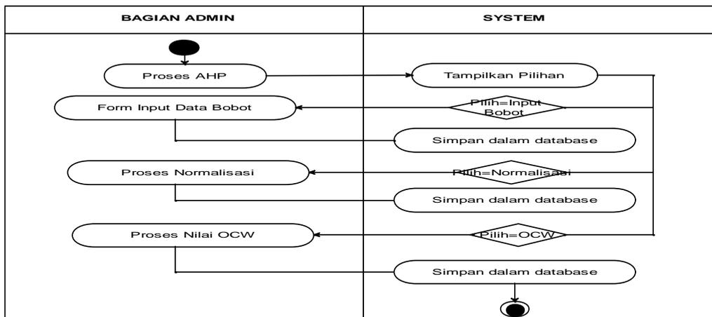
Gambar 7. Activity diagram proses ahp
